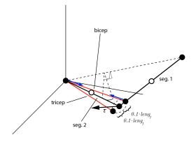
Each muscle is treated as a tension between two fixed endpoints.
