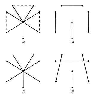
FIG. 8. Worst-case example for V-join or matching. Graph (a) gives the instance: plain edges have cost 1, dotted edges have cost  $1 + \epsilon$ , and all other edges have cost 2. Graph (b) is the minimum-cost solution. Graph (c) is the set of edges found by the constrained forest algorithm, and graph (d) shows a bad (but possible) shortcutting of the edges to a matching.
